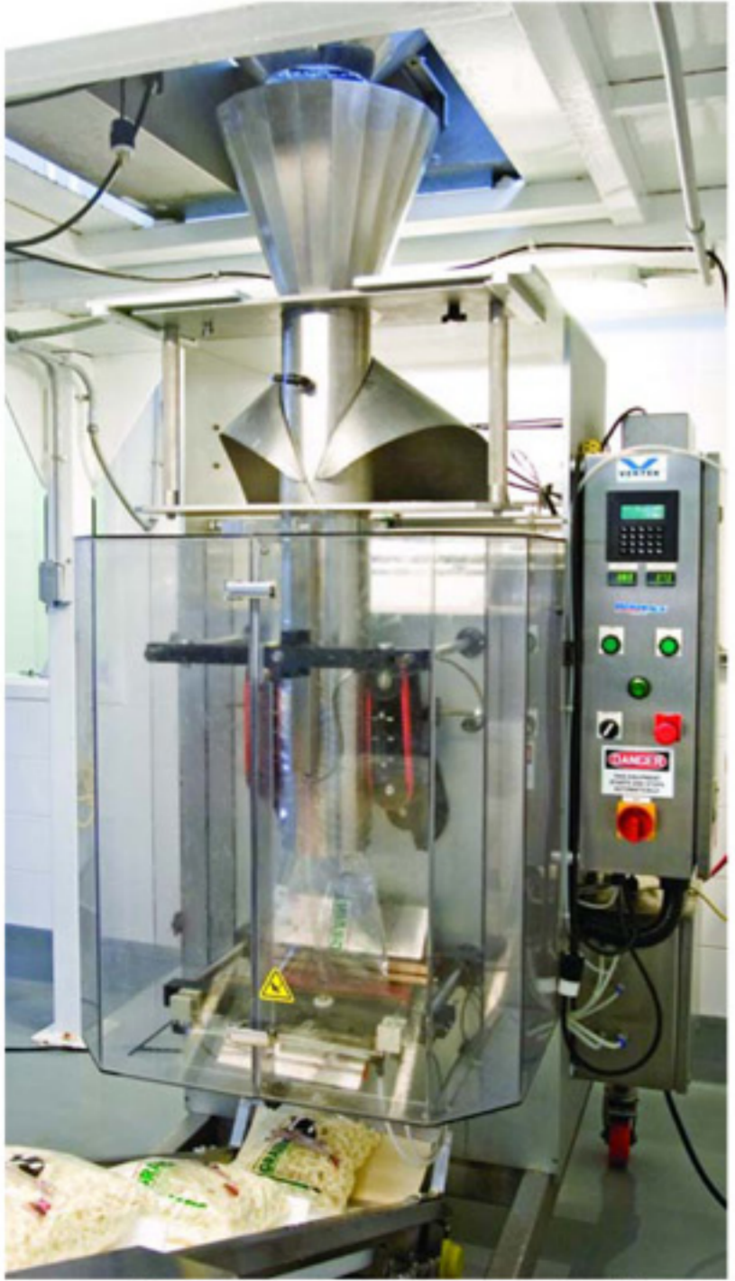
A Vertek 1150 automatic bagger is capable of filling and sealing plastic bags at rates of up to 45 bags a minute.
