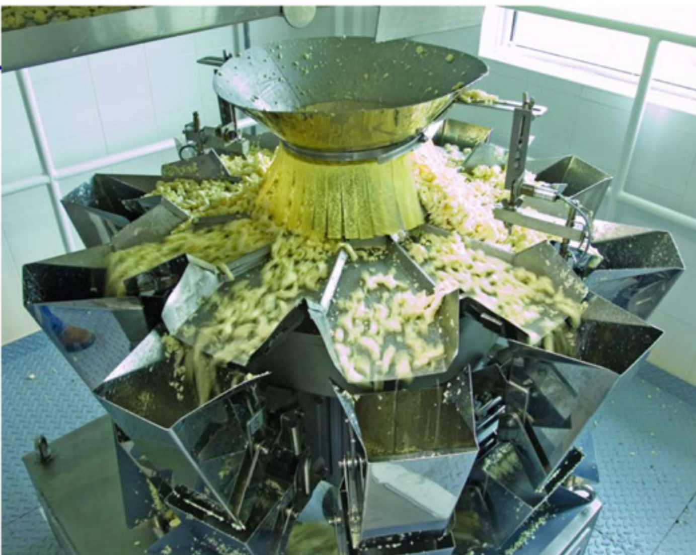
The 10-head WeighPack CombiScale at Champetre can fill over 100 packages of cheese curds per minute, and it is accurate to the gram.
