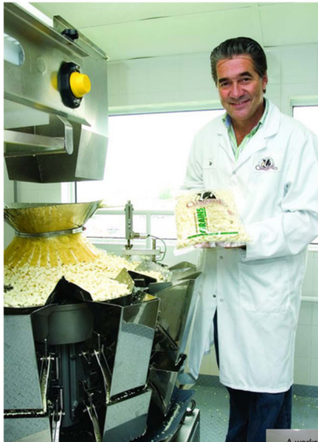
Luc Livernoche, president of La Fromagerie Champêtre, holds up a bag of freshly-packaged cheddar-cheese curds in front of the WeighPack CombiScale weighing and filling machine.
