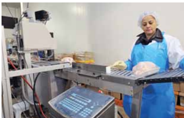
Trays of product move past a Markem-Imaje inkjet coder to have lot data and product codes applied.
