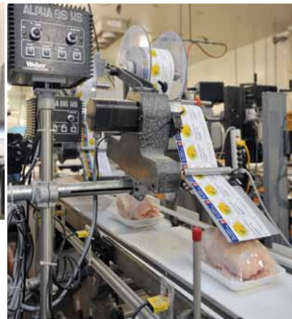
An Alpha 86 HS labeler, from Weber ensures quick and precise label placement onto the passing packages.
