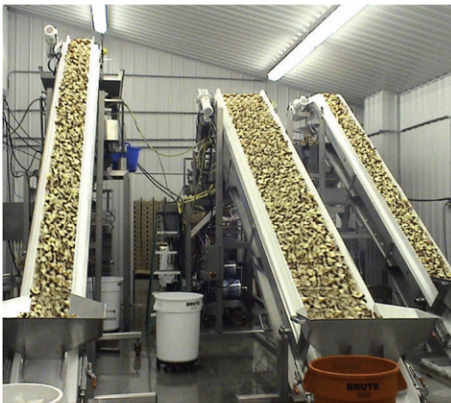
[above] An incline infeed conveyor carries the sliced fruit (in this case apples) to a CombiScale14 Head Combination scale.
