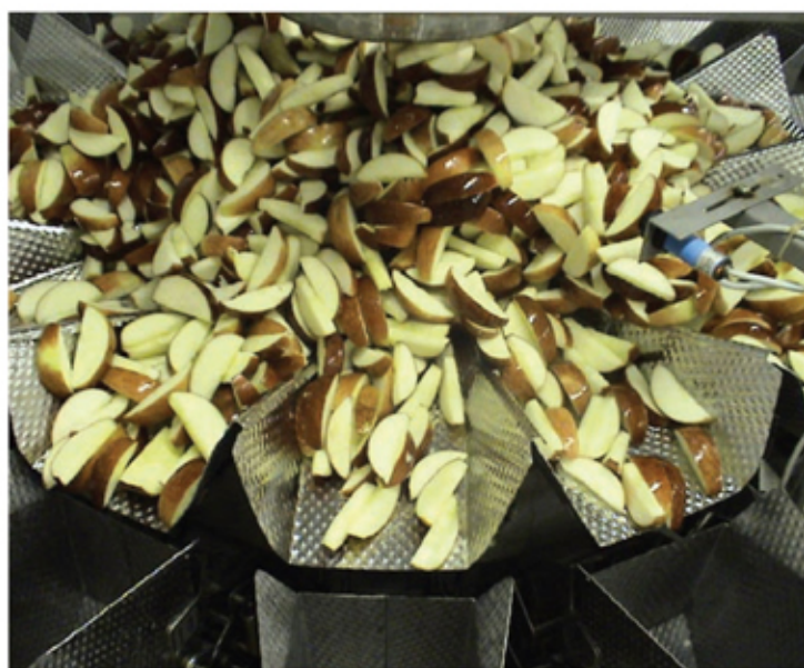
[right] The scale is able to accurately weigh 58-gram bags within one gram.
