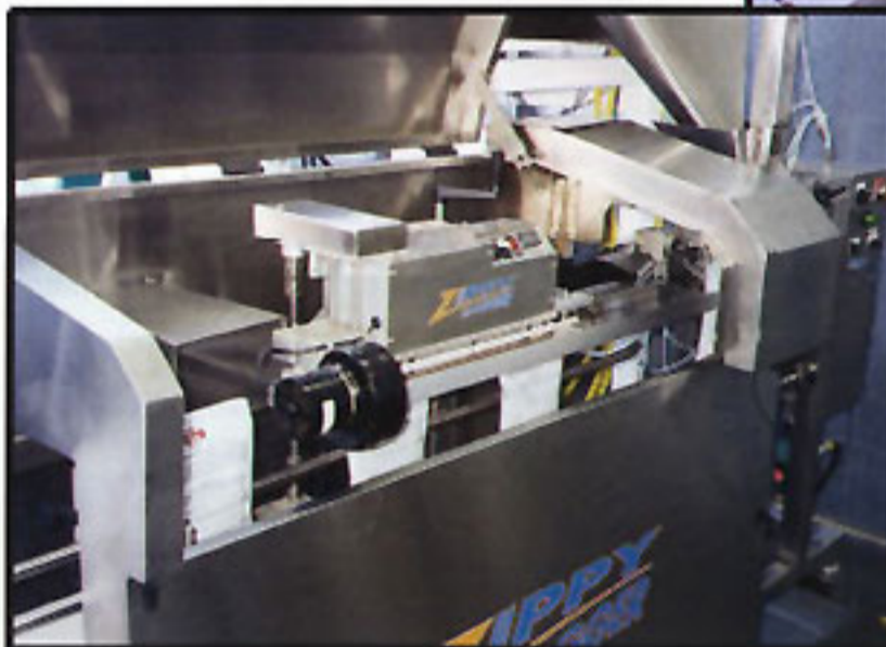
Weigh/fill/bagging system, top left, has an accuracy of +/- 1 gram (300 seeds). As the bag leaves the heating section, it passes a rotary cutter, left, that removes the plastic material above the seal. To start each fill cycle, an air jet blows downward to open the top of the bag, above, after which a plunger descends to completely open the bag plus "pop out" the bottom gusset.
