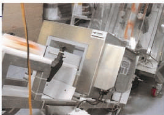
An inline Fortress metal detection system doing final quality control inspection on the passing 500-gram bags of frozen perogies.
