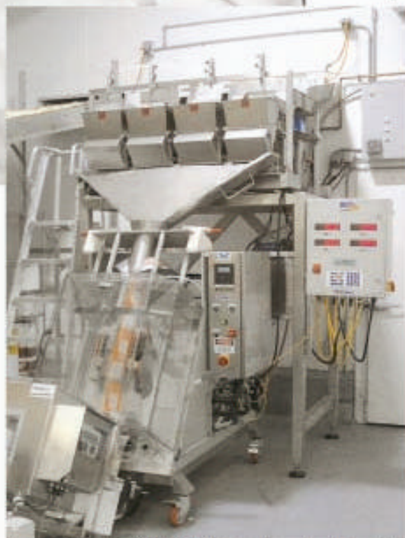
The recently-installed WeighPack VFFS machine and related packing equipment enable Supreme to bag up to 35,000 perogies per hour.
