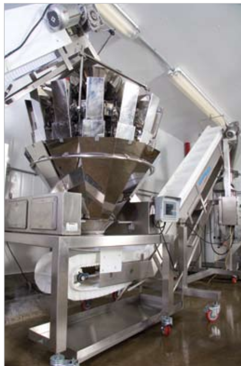
The 14-head CS-145B CombiScale multihead scale ensures weighing accuracy to within one gram.
