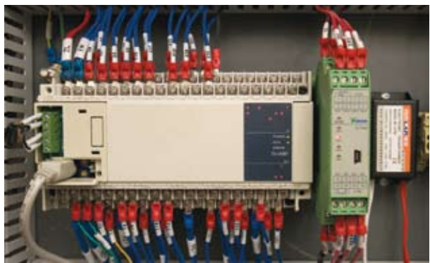
A large Omron PLC (programmable logic controller) controls the WeighPack XPdius 1200 machine's forming, filling and sealing operations.
