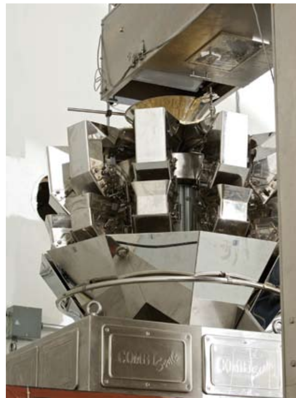
The high-speed, 10-head CombiScale weigher owned by Snack Brands can perform up to 80 high-precision measurements per minute.
