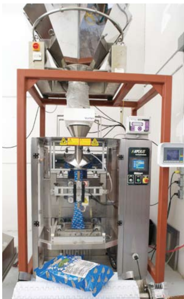
Snack Brands purchased an XPdiius 1200 vertical form/fill/seal bagger with a CS-10 SB CombiScale from WeighPack Systems Inc. with the optional date-coder and a gas-flushing system, helping the gourmet popcorn manufacturer obtain dramatic reductions in its labor costs.
