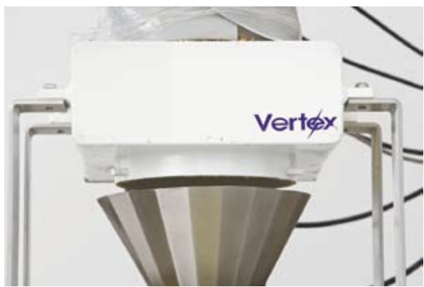
A Vertex Phantom Series metal detector from Fortress Technologies is used to catch any unwanted particles in the free-flowing product.
