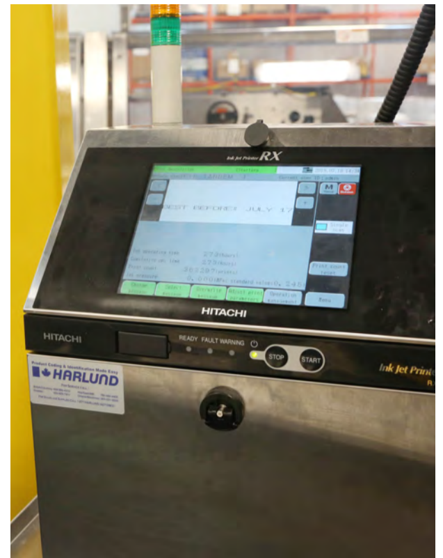
Schep's Bakery uses a Hitachi small-character inkjet printer supplied by Harlund Industries to apply barcodes and other key product data onto the finished stroopwafel product.
