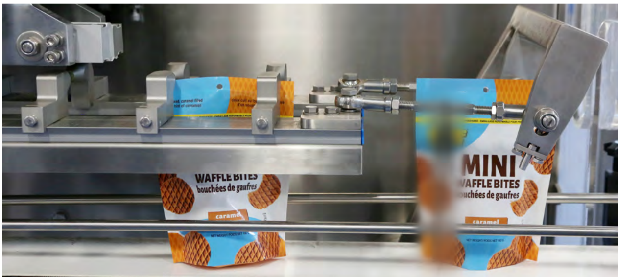
The mini stroopwafel products are sealed thanks to the Swifty Bagger 3600 (See Sidebar).
