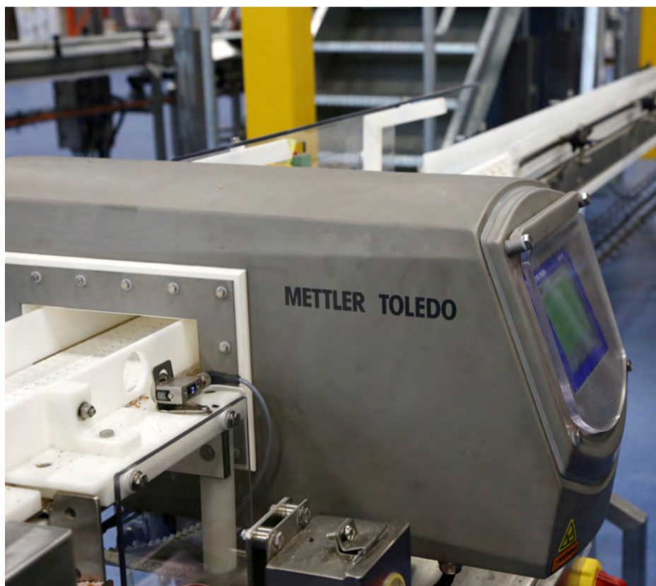
The waffle cookies are run through a METTLER TOLEDO metal detection system to check for any possible contaminants that may have inadvertently made their way into the product before being distributed for retail sale.
